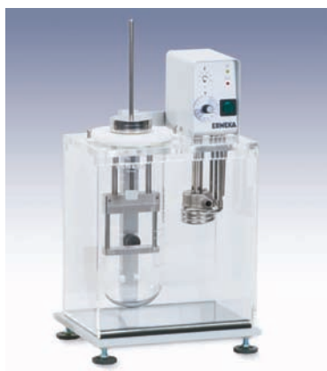
Suppository Hardness Tester, type SBT 2.
