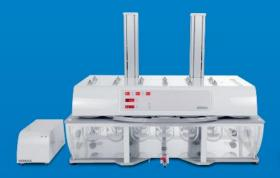
The DT 1412 with 12 test stations can also be configured as an UV/ VIS On-/Offline system. This configuration has an ASS-14 autosampling station on top of the tester and an IPC-16 pump which connects to an ERWEKA SPM 16 or an Analytic Jena Specord 210/16 with two cuvette changers and FRL 624-2 sample collector, all managed via PC and ERWEKA Dissolvet software.
