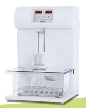
The ERWEKA ZT 220 series is available with 1, 2, 3 or 4 test stations, driven by one synchronic motor. Each test station is operated in a separate glass vessel, which are placed in the PET moulded bath with cover to minimize evaporation.
