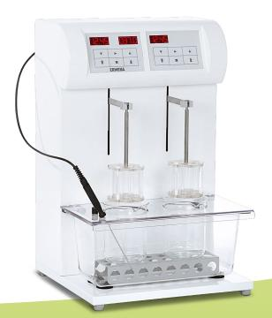
The ZT 320 series comes with 1, 2, 3 or 4 individually operated test stations controlled by a dedicated keypad per station for easy setting of the required run-time parameters as well as start/stop operation.
