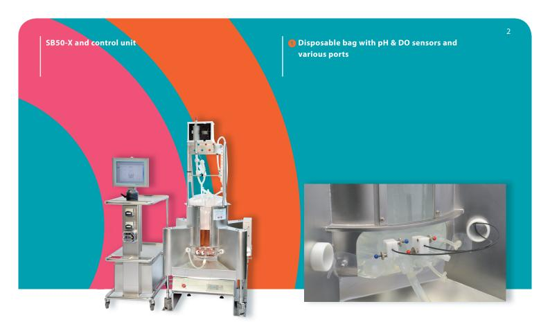
The SB50-X is an orbital shaken bioreactor for the cultivation of human, mammalian and plant cells in a disposable bag. A working volume from 15 litres up to 50 litres for the SB50-X ensures easy scale-up from microtiter plates to shaking flasks and all the way up to 200 litres. The SB50-X can be used in research, process development or production.
